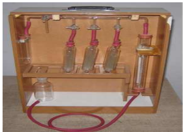
5.3 Diagram of ORSAT apparatus
